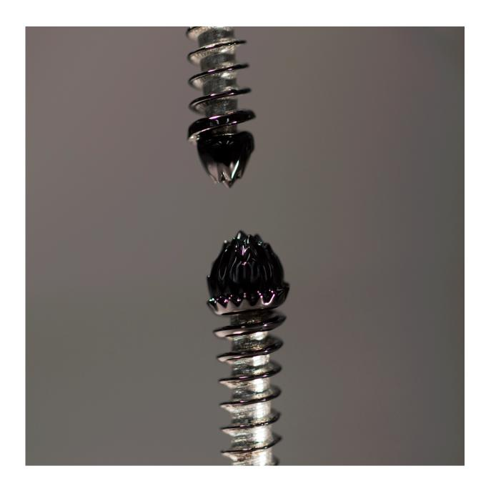
Without a magnetic field, ferrofluids look like a tarry, oil-based fuel. With a magnetic field, the propellant self-assembles, raising into a spiky ball. Credit:
