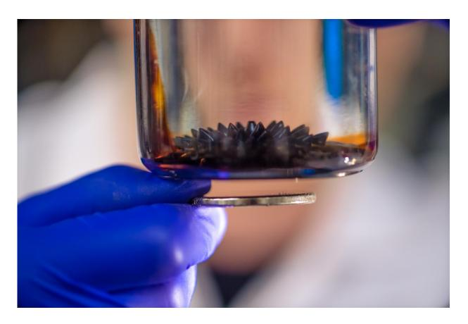
A ferrofluid is a magnetic liquid that turns spiky in a magnetic field. Add an electric field and each needle-like spike emits a jet of ions, which could solve micropropulsion for nanosatellites in space. Credit: Sarah Bird/Michigan Tech
