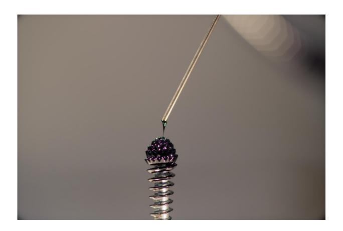
A ferrofluid is a magnetic liquid that turns spiky in a magnetic field. Add an electric field and each needle-like spike emits a jet of ions, which could solve micropropulsion for nanosatellites in space. Credit: Sarah Bird/Michigan Tech
