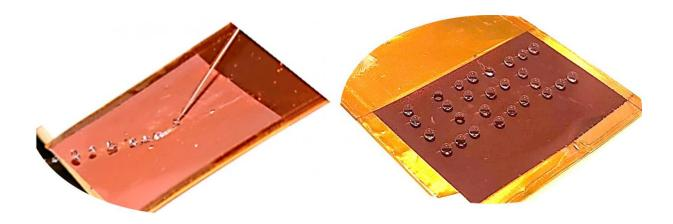
UBC-developed smart surface offers fast and reversible surface wetting properties-from superhydrophobic (water-repellant) to superhydrophilic (waterattractive) using a small voltage that could be supplied by conventional batteries. Credit: University of British Columbia
