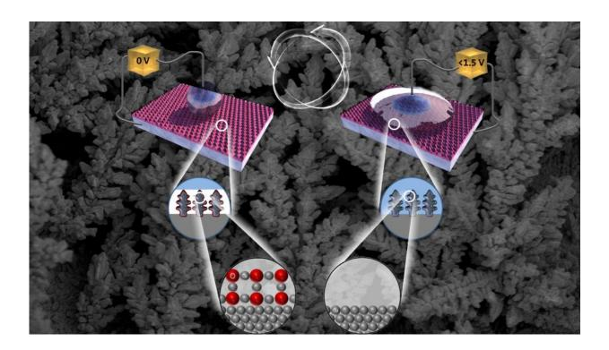
Applying low voltage to a nanostructured copper surface changes its oxidation state, and hence its ability to attract and repel liquids. Credit: University of British Columbia
