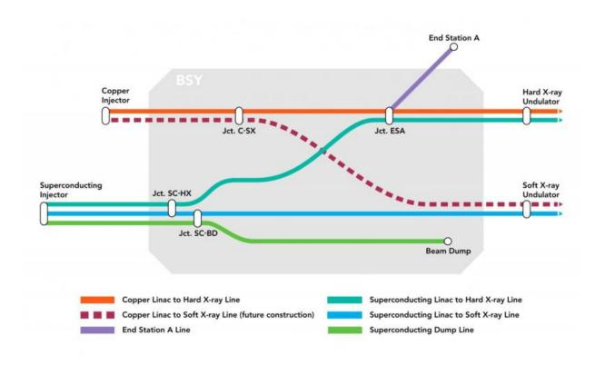
A reconfiguration of SLAC's historic Beam Switch Yard will include electron transport lines needed for LCLS-II, a major upgrade to the Linac Coherent Light Source (LCLS) X-ray laser. Credit: Greg Stewart/SLAC National Accelerator Laboratory
