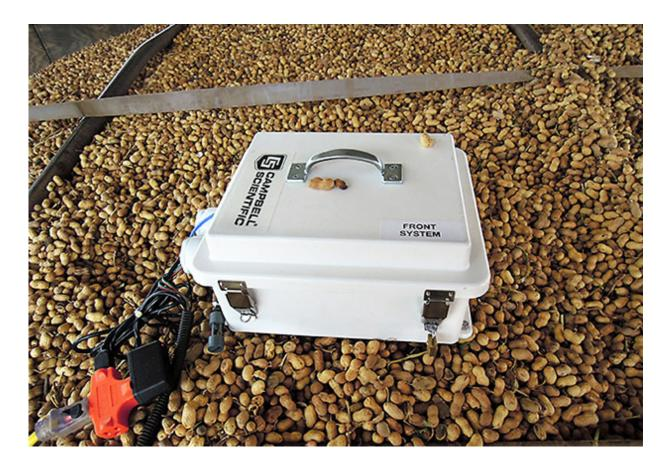
ARS scientists developed a new moisture-monitoring system for use in peanutdrying trailers. Credit: Samir Trabelsi
