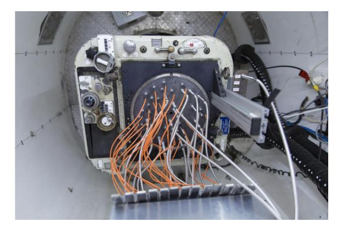
The SAMI instrument at the 3.9m Anglo-Australian Telescope. Each silver "cable" has a "hexabundle" that allows it to dissect an object. The orange fibres are used for calibration purposes. Credit: Ángel R. López-Sánchez
