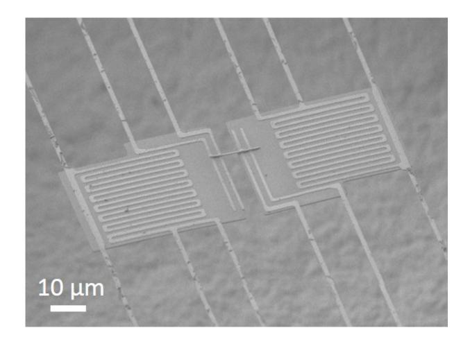
SEM images of suspended micro-island devices. Individual AIHP NW is suspended between two membranes. Credit: UC Berkeley
