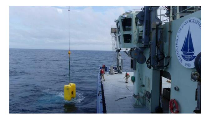
The crew aboard the R/V Neil Armstrong helps guide Clio into the water for tests at sea. During the expedition, Clio completed five dives, including two dives to 2,000 meters (1.2 miles), and filtered more than 1,000 liters (264 gallons) of se awater from nine different depths. Credit: Mak Saito, Woods Hole Oceanographic Institution
