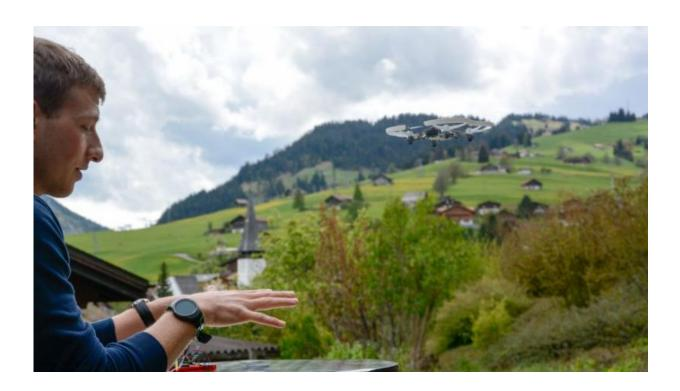
The watchstrap contains piezoresistive fibers produced on a 3D printer. The wrist movements are transmitted to steer the drone. Credit: Swiss Federal Laboratories for Materials Science and Technology
