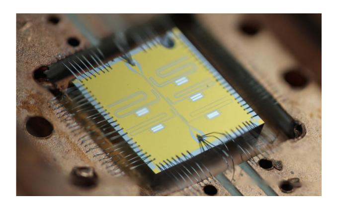
A multi-qubit chip developed in the Quantum Nanoelectronics Laboratory at Lawrence Berkeley National Laboratory.
