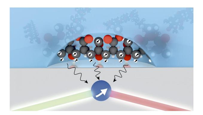
A nitrogen-vacancy (dark blue) quantum probe in diamond (light grey) performing nanoscale nuclear magnetic resonance (NMR) on molecular hydrogen sitting on the diamond's surface. A green laser controls the quantum state of the probe, which is tuned to the resonant frequency of target nuclear spins. The probe responds to the nuclear spins of the hydrogen atoms and provides a direct measurement via the red light emitted. Credit: David A. Broadway/cqc2t.org
