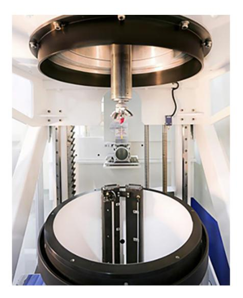
Researchers will image the crystal structure of the AChE protein crystals grown in space on the IMAGINE sample station at Oak Ridge National Laboratory. Credit: DOE
