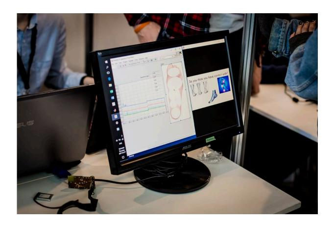
It records the data from mobile sensors placed on an insole of a shoe. Later, it is being sent via Bluetooth connection to a computer for visualization. Credit: KTU
