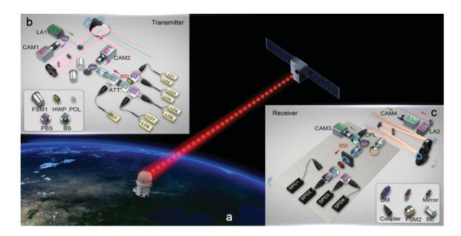
Illustration of the experimental set-up from "Satellite-to-ground quantum key distribution" arXiv:1707.00542 [quant-ph]
