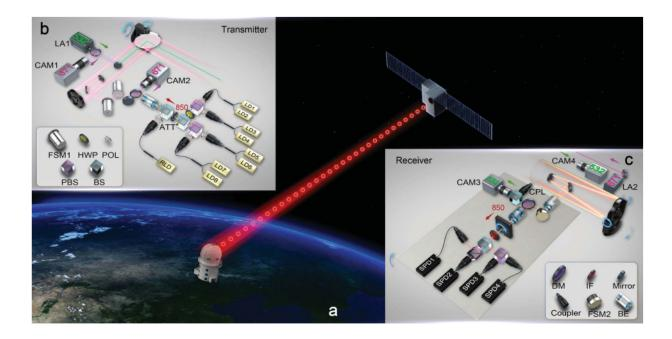
Illustration of the experimental set-up from "Satellite-to-ground quantum key distribution" arXiv:1707.00542 [quant-ph]
