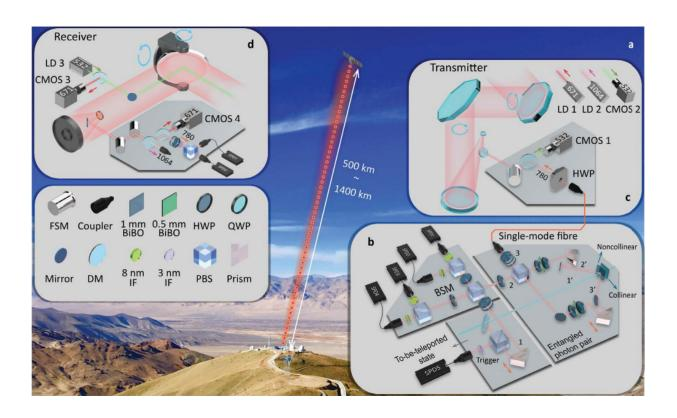
Overview of the set-up for ground-to-satellite quantum teleportation of a single photon with a distance up to 1400 km. Credit: arXiv:1707.00934 [quant-ph]
