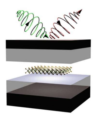
Schematic showing control of valley properties in 2-D semiconductors embedded in microcavity. Credit: Zheng Sun
