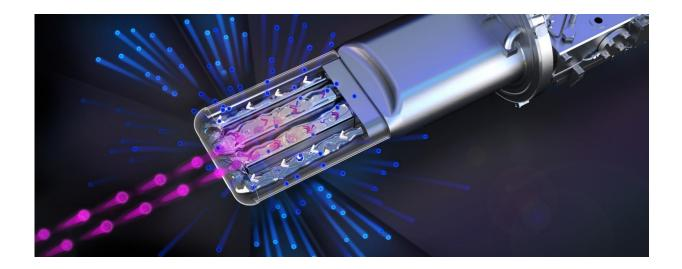
As the proton beam (pink) impinges upon the target and passes into the liquid mercury inside, the mercury absorbs the protons and creates a "spall" of neutrons (blue) that are then sent through moderators and guides to research instruments to study the fundamental properties of materials. Credit: ORNL/Jill Hemman
