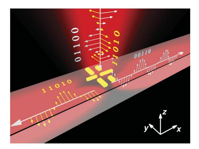
Scheme of a waveguide-integrated plasmonic nanoantenna for mode-selective polarization (de)multiplexing. The device couples light of orthogonal polarizations into different directions and modes of the underlying silicon waveguide. Credit: *Science Advances* (2017). DOI: 10.1126/sciadv.1700007
