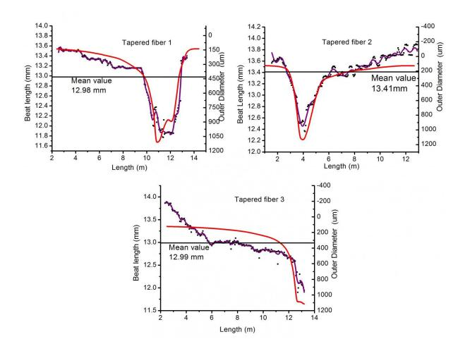
Fig. 3. The polarization beat length (the violet curve on the left axis) and the outer cladding diameter (the red curve on the right axis) along the length of the fiber samples Credit: MIPT
