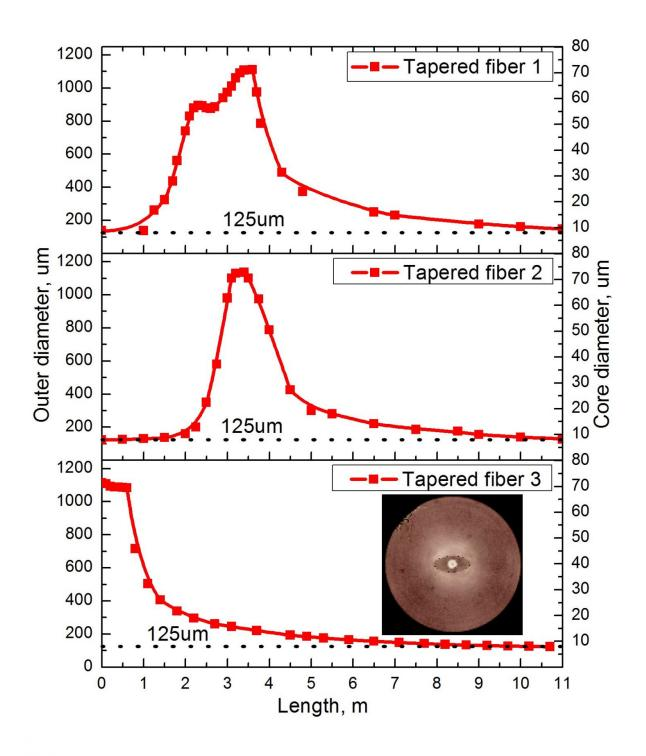
Fig. 2. The diameter of the outer cladding (on the left axis) and the core (on the
