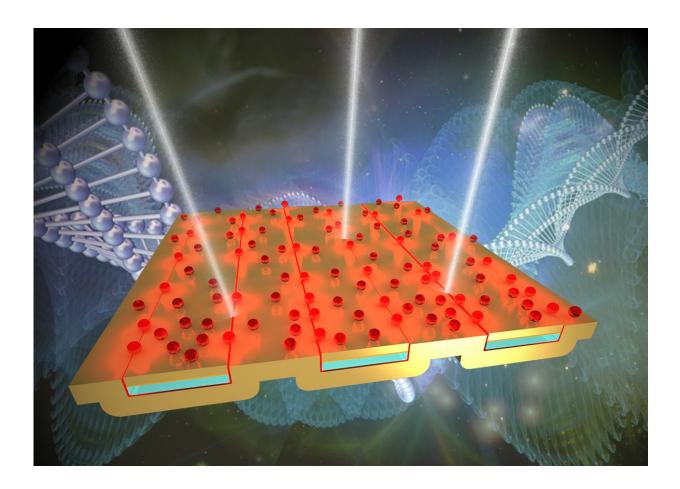
The image depicts a new device for surface enhanced infrared absorption spectroscopy. Infrared light (the white beams) is trapped by tiny gaps in the metal surface, where it can be used to detect trace amounts of matter. Credit: University at Buffalo
