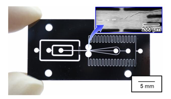
The photograph shows the developed microfluidic chip which enables us to sort cells at high speed of 16 microseconds. The enlarged view shows a demonstration of on-chip cell sorting of a Euglena gracilis cell (time interval of each frame: 40  $\mu$ s). © Shinya Sakuma, Yusuke Kasai, Takeshi Hayakawa, and Fumihito Arai . Credit: Nagoya University
