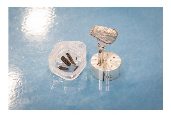
The ORNL-led research team selected a crystal composed of copper bromide -because the copper ion is ideal for studying exotic quantum effects -- to observe the elusive Higgs amplitude mode in two dimensions. The sample was examined using cold neutron triple-axis spectrometer beams for neutron scattering at the High Flux Isotope Reactor. Credit: Genevieve Martin, Oak Ridge National Laboratory/Dept. of Energy
