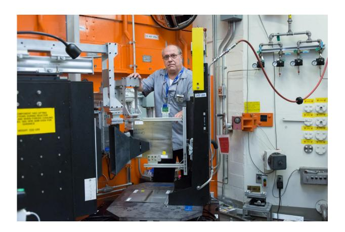
Daryush Aidun uses HFIR beam line HB-2B to study a dissimilar weldment of low carbon steel and stainless steel, measuring where and how residual stresses are distributed within the structure. Credit: ORNL/Genevieve Martin
