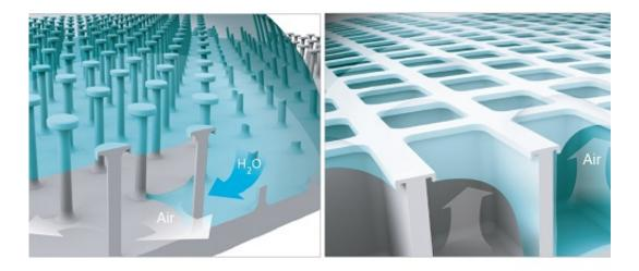
Wetting surfaces with micropillars (left) lose their omniphobicity when damaged, while microtextures with doubly reentrant cavities (right) exhibit omniphobicity despite localized damage. Reproduced with permission from ref 1.© 2017 American Chemical Society. Credit: Ivan Gromicho © 2017 KAUST
