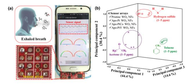
Demonstration of mobile breath analysis using a portable sensing module. (a) Low-power sensing of simulated biomarker using MEMSsensor arrays and (b) pattern recognition of H2S, acetone, and toluene using PCA. Credit: KAIST
