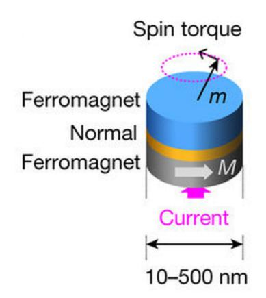
Schematic of a spin-torque nano-oscillator, consisting of a non-magnetic spacer (gold) between two ferromagnetic layers, with magnetization m for the free layer (blue) and M for the fixed layer (silver). A current injected into the oscillator induces magnetization precessions of m. For our experiments we used a nano-oscillator with a diameter of 375 nm; however, diameters of 10–500 nm are possible. Credit: *Nature* (2017). DOI: 10.1038/nature23011
