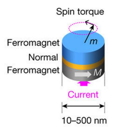
Schematic of a spin-torque nano-oscillator, consisting of a non-magnetic spacer (gold) between two ferromagnetic layers, with magnetization m for the free layer (blue) and M for the fixed layer (silver). A current injected into the oscillator induces magnetization precessions of m. For our experiments we used a nano-oscillator with a diameter of 375 nm; however, diameters of 10–500 nm are possible. Credit: *Nature* (2017). DOI: 10.1038/nature23011
