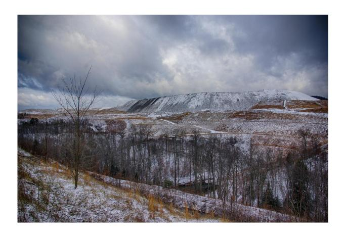
A portion of the Hobet 21 coal mine in West Virginia shows the effects of mountaintop-removal mining, which, new research shows, causes many streams and rivers in Appalachia to run consistently saltier for up to 80 percent of the year. Credit: Fabian Nippgen
