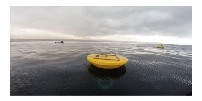
Buoys float off the coast of Ilo, Peru, in a 2015 test of a wave energy system developed by the Santa Fe, New Mexico, company Atmocean with technical help from Sandia National Laboratories. The system powers a desalination plant that provides coastal cities with fresh water. Credit: Atmocean Inc.
