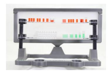
Prototype of the Capillary Evaporator hardware comprised of a test stand, lighting backdrop, and test arms to hold transparent capillary structures filled with test fluids. The structures are photographed over the course of several days while the fluids evaporate. Credit: IRPI LLC
