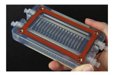
The Capillary Sorbent contactor designed with parallel, open channels to expose liquid to ambient air while containing and wicking fluids in a controlled manner. Credit: IRPI LLC
