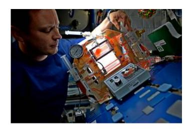
NASA astronaut Jack Fischer works with the capillary sorbent hardware, that is made up of 3-D printed contactors (center) with several capillary channels. The contactors, or capillary structures under investigation, are supported by tubing, valves, and a pump. This highly interactive experiment simulates the fluidics of a liquid sorbent system for the removal of CO2 from the air. Credit: NASA
