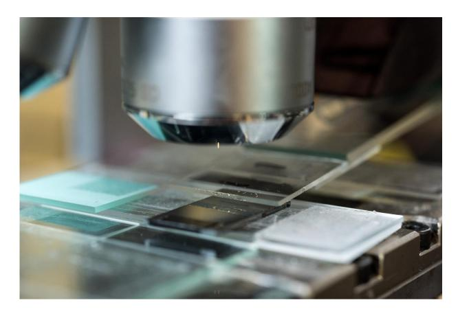
Samples produced by the meniscus-assisted solution printing (MASP) technique are studied under this optical microscope. Credit: Credit: Rob Felt, Georgia Tech
