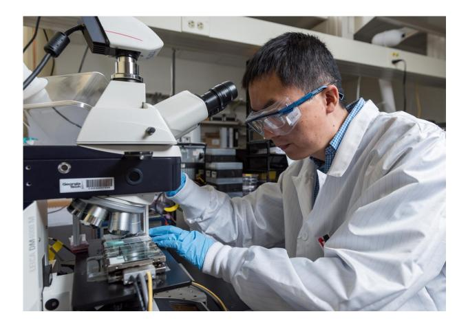
Georgia Tech Research Scientist Ming He adjusts the equipment for the meniscus-assisted solution printing (MASP) technique used to fabricate perovskite films for solar cells. Credit: Credit: Rob Felt, Georgia Tech
