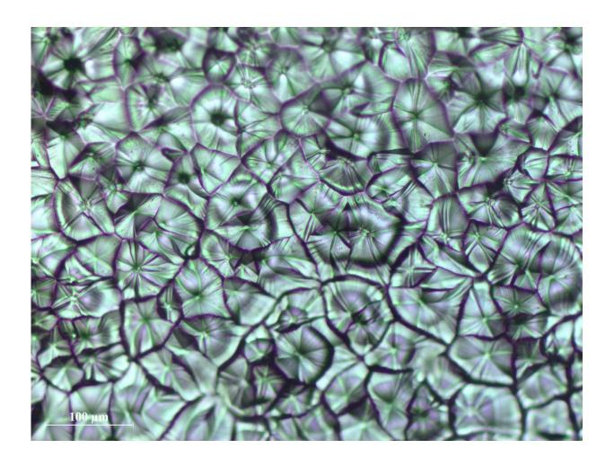
Optical micrograph of perovskite crystal grains crafted by meniscus-assisted solution printing. Credit: Ming He, Georgia Tech
