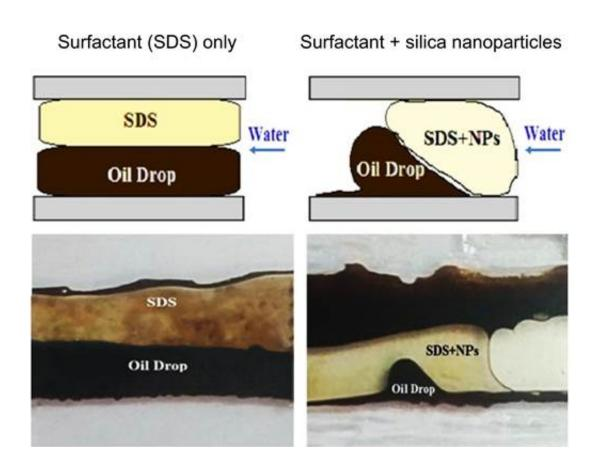
Differences of the movement of oil through the micro channels of the addition of surfactant in the presence of silica nanoparticles as compared to the surfactant alone showing how the nano-sand alters the extraction of the oil. An effective formula for EOR applications, according to the scientists at Swansea University. Credit: Goshtasp Cheraghian /Azad University/Iran
