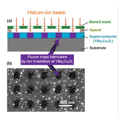
The principle of the fabrication of a "quantum egg-box" with a novel masked ion-beam technology, developed by the researchers. It allows to produce at the same time hundreds of thousands of traps for fluxons, magnetic flux quanta, in a superconductor. The picture at the bottom shows an electron-microscope image of the surface of the superconductor with some of these traps. Credit: Copyright: Wolfgang Lang, University of Vienna
