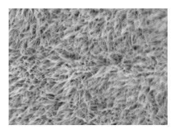
Nickel cobalt oxide nanowires — less than 100 nanometers across and roughly 3.5 micrometers long — boost the performance of the hybrid zinc battery. Credit: A\*STAR Institute of Materials Research and Engineering
