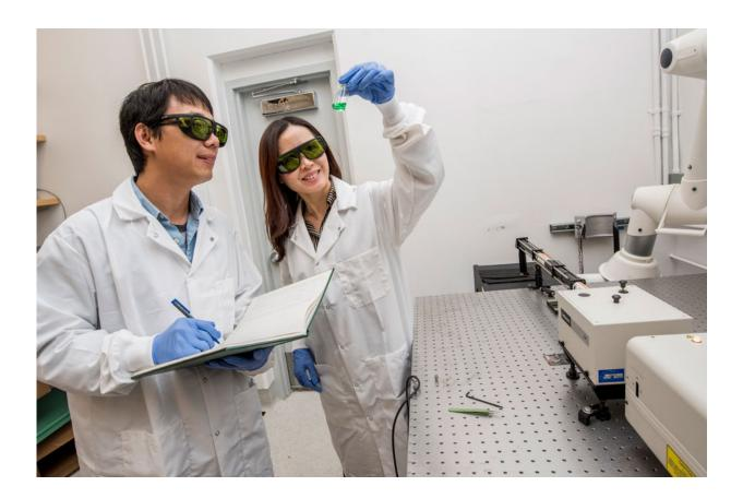
Berkeley Lab scientists Kaiyang Niu (left) and Haimei Zheng, principal investigator, developed a new photocatalyst of metal organic composites that can effectively convert carbon dioxide into the ingredients for fuel. They made the new material, held by Zheng in a glass vial, by exposing a precursor solution to laser irradiation. Credit: Marilyn Chung/Berkeley Lab
