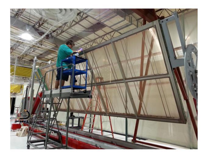
Physical Sciences Laboratory electronics technician Andy Arbuckle soldering 150 micron CuBe wire on the anode panel assembly (APA). Four underground detector modules in South Dakota will each be two-thirds the size of a football field and comprise 150 APAs. Credit: UW-Madison Physical Sciences Laboaratory
