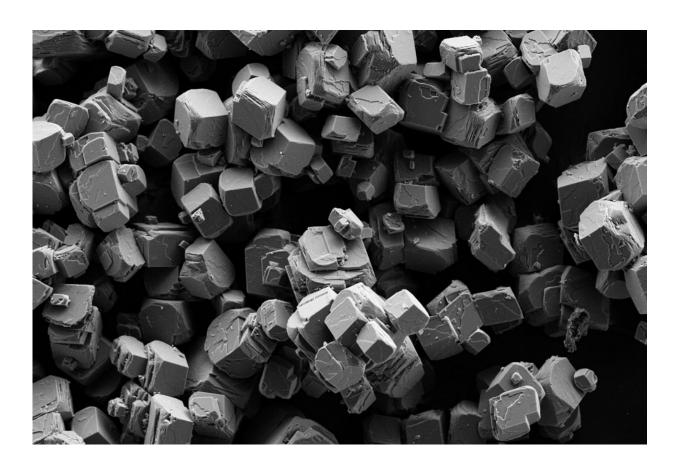
Scanning electron microscopy image of calcite. Credit: Adam Subhas/Caltech
