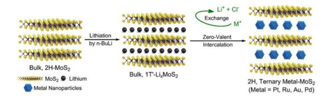
Figure 1: The encapsulation of noble metal nanoparticles in MoS2 by an in-situ reduction strategy.
