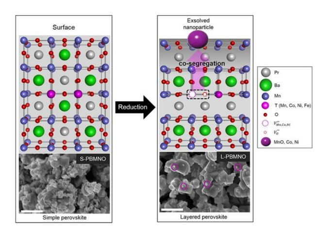
Exsolution of B-site cation with oxygen from layered perovskite in a reducing atmosphere. Credit: UNIST
