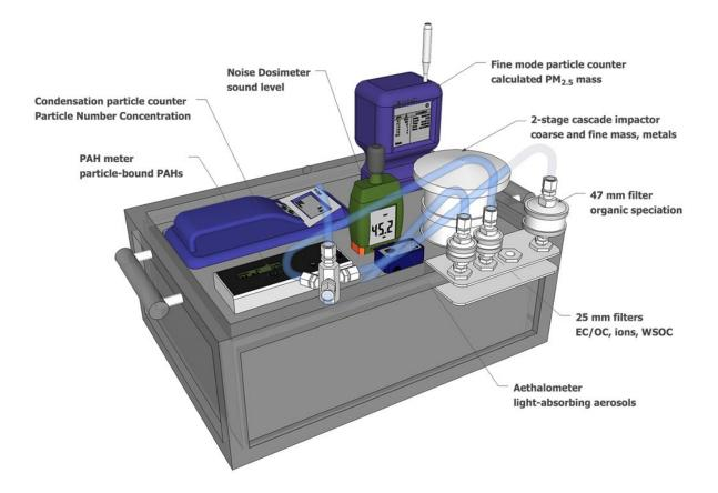
A schematic of the sampling device built by researchers to measure levels of toxic particulate matter present during rush hour inside of a typical car cabin. Credit: Heidi Vreeland, Duke University
