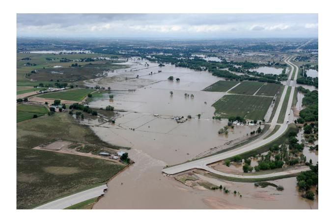
This picture was taken above Greeley, Colo. on Sept. 16, 2013. As a result of the flooding, the state lost approximately 500 miles of roadway and more than 30 bridges. Here, U.S. 34 in Greeley is breached by the South Platte River in flood stage. Credit: US Environmental Protection Agency
