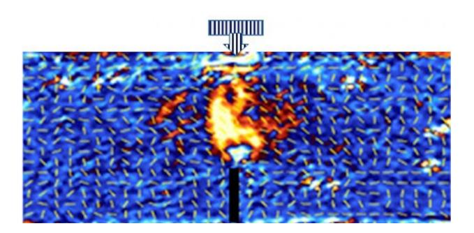
A picture from a photonic camera showing how using the coating can create a candle-like 'flame' highlighting shear stress distribution in a sample concrete beam. Credit: University of Leeds
