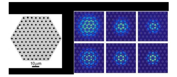
Fig. 4: Image of the microstructure of a coreless t-PCF recorded with a scanning electron microscope. The axis of rotation roughly coincides with the hollow channel at the centre. (b) Experimental (top) and calculated (bottom) normalized intensity distributions for 818 nm for three different twisting rates. Credit: MPI for the Science of Light
