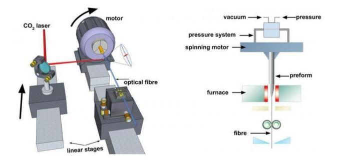
Fig. 2: Manufacturing process for t-PCF. (a) Thermal post-processing with a carbon dioxide laser. The laser travels over the fibre, thereby heating it up to its melting point, while one end of the fibre is twisted by the motor and the other is held tight. (b) Rotating glass preform as the fibre is being drawn in the fibre-drawing tower. Credit: MPI for the Science of Light
