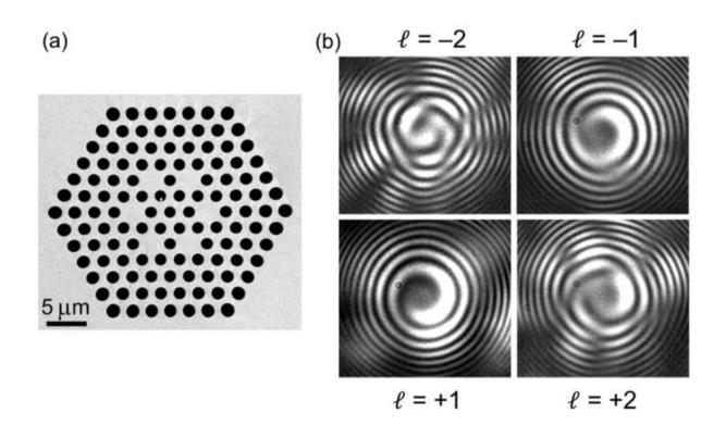
Fig. 3: Image of the t-PCF with six satellite cores recorded with a scanning electron microscope. The twisting rate  $\alpha$  is 2.9 rad/mm. (b) Experimentally recorded helical patterns which arise when modes with different orders of main orbital angular momentum  $\ell$  interfere with a diverging Gauss beam after they have propagated in the t-PCF. Credit: MPI for the Science of Light
