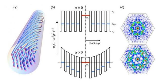
Fig. 1: (a) Sketch of a twisted single solid core PCF. (b) Top: Cross-section through the distribution of the refractive index of an untwisted (top) and a twisted (bottom) solid core PCF (schematic). The increase in the optical path length along the helical path increases the effective refractive index according to the factor  $(1+\alpha 2\rho 2)1/2$  (c) Two examples of ring modes. Credit: MPI for the Science of Light
