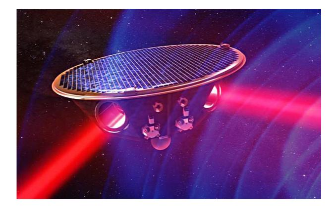
The proposed LISA mission will detect gravitational waves in space using a trio of satellites, separated by millions of kilometers. Lasers will be employed to measure the minute changes in their relative distance induced by impinging gravitational waves. Credit: AEI/MM/exozet; GW simulation: NASA/C. Henze
