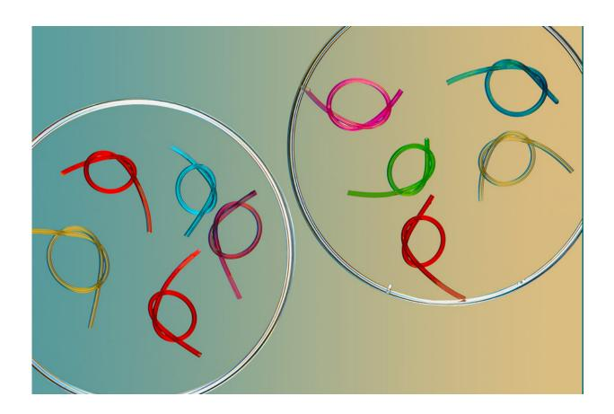
MIT engineers have designed a gel-like material that can be coated onto standard plastic or rubber devices, providing a softer, more slippery exterior that can significantly ease a patient's discomfort during surgery. Credit: Felice Frankel
