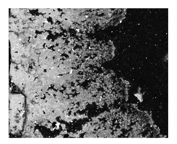
Back scattered electron images of a cross-section of the layer of metal scale, or rust, inside pipe samples from lead service lines in Flint, Michigan. The outside of the pipe is on the left side, and the holes in the "Swiss cheese pattern" are voids where the lead used to be, say researchers at the University of Michigan
