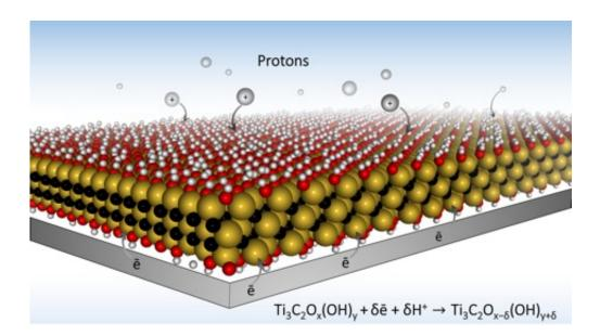
Drexel University researchers have developed two new electrode designs, using MXene material, that will allow batteries to charge much faster. The key is a microporous design that allows ions to quickly make their way to redox active sites. Credit: Drexel University
