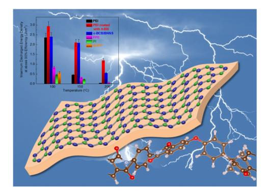
PEI coated with hexagonal boron nitride (hBN) nanosheets significantly outperforms competitive polymers at operating temperatures needed for electric vehicles and aerospace power applications. Credit: Feihua Liu/ Penn State
