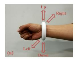
(Left) Broken-out sectional view of the energy-harvesting bracelet, in which magnets moving through copper coils generate a voltage. (Right) Photo of the bracelet. Credit: Wu et al. ©2017 American Institute of Physics
