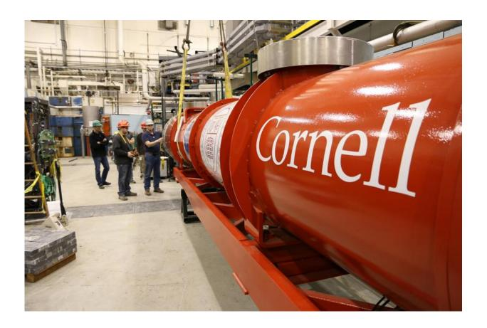
Main linac cryomodule being placed into its final position by Cornell Engineers at Wilson Lab. Credit: Cornell University
