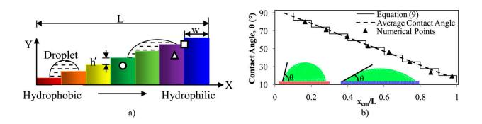
(a) Schematic representation of the simulation domain for a droplet climbing the stepped surfaces under the effect of differential wettability, O: trailing step,  $\Delta$ : leading step, and  $\square$ : foot of the step, and (b) comparison of applied and numerically obtained contact angles. Credit: *Physics of Fluids* (2017). DOI: 10.1063/1.4985213
