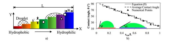
(a) Schematic representation of the simulation domain for a droplet climbing the stepped surfaces under the effect of differential wettability, O: trailing step,  $\Delta$ : leading step, and  $\Box$ : foot of the step, and (b) comparison of applied and numerically obtained contact angles. Credit: *Physics of Fluids* (2017). DOI: 10.1063/1.4985213
