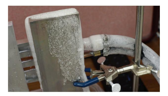
Boreyko, along with undergraduate students William McClintic and Kevin Murphy, experimented by treating aluminum plates to render them superhydrophobic -- that is, so water-repellent that droplets easily roll off without sticking to the surface. Credit: Virginia Tech
