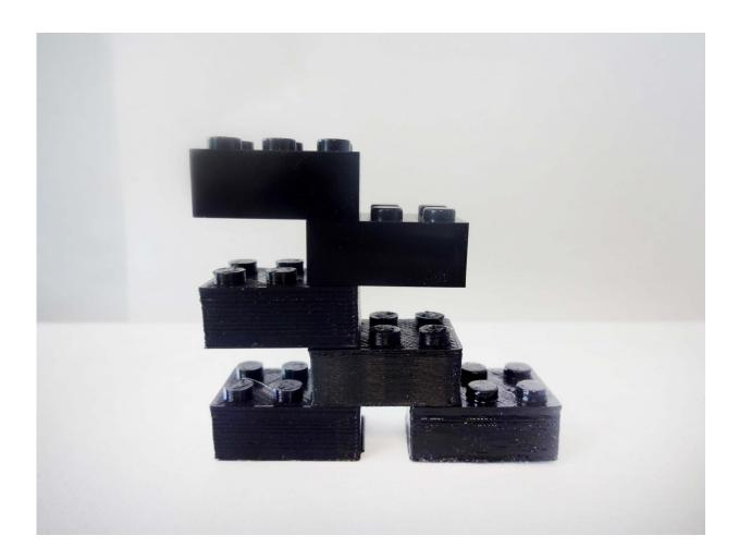
Each plastic building block is made of a different plastic and process; 3-D printing has the potential to disrupt conventional toy production, making it cheaper to make toys at home. Credit: Joshua Pearce
